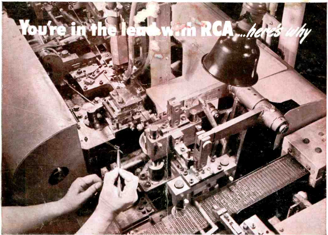
Automatic high-speed getter machine operation—a tube manufacturing technique pioneered by RCA.
